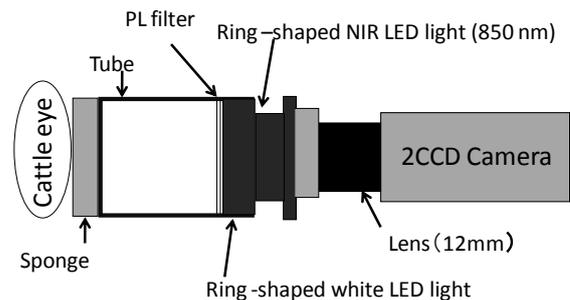
Fig. 3 Sketch of experimental device.
