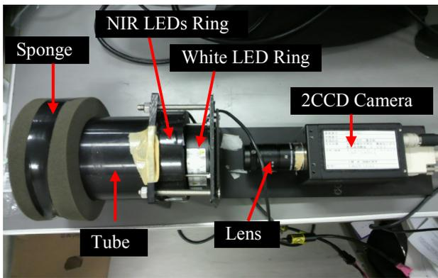
Fig. 2. Appearance of the device
