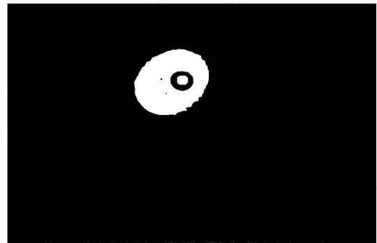
Fig. 7. Binarized image after the salt-and-pepper noise reduction (pupil detection)
