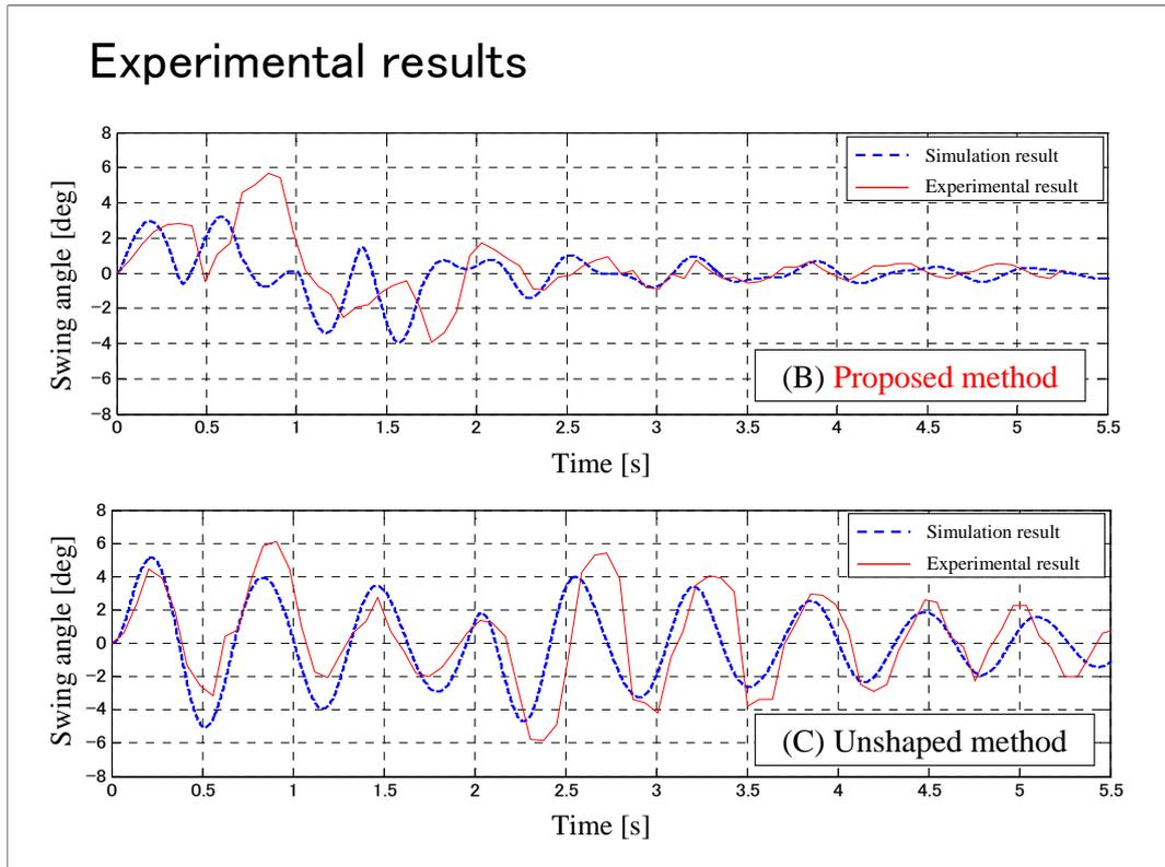
Here is experimental results with simulation results. Red line is experimental result and blue dot line is simulation result. Both results are very similar after end-effector stopped.
