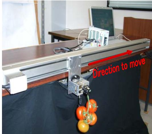
We conduct an experiment to compare the methods as well as the simulation. Here, these two methods were actually compared by use of this 1 DOF manipulator.
