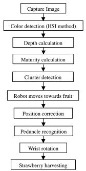
Fig. 3 General flow of the harvesting process
