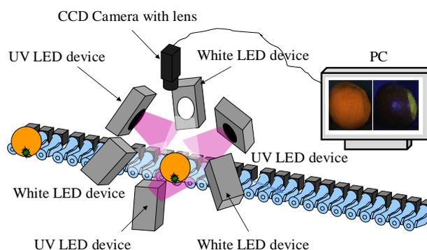
Fig. 1 Layout of the double LED image acquisition system
