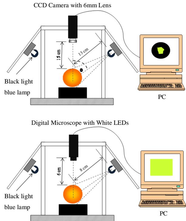
Fig. 4 Schematic representation of UV (up) and Digital Microscope image acquisition systems (bottom)
