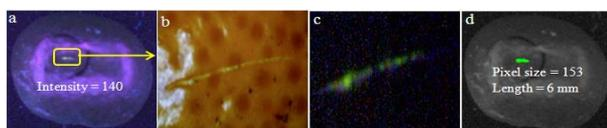
Fig. 6 Examples of thin scar fluorescence area: (a) fluorescence image captured by UV illumination, (b) and (c) color and fluorescence images of fluoresced areas captured by digital microscope, (d) processed fluorescence image
