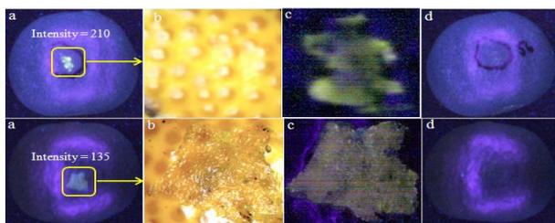
Fig. 9 Examples of fluorescence caused by contact with decayed fruit
