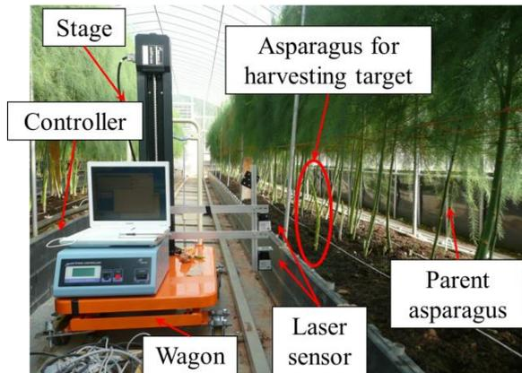
Fig. 3 Equipment for detecting asparagus
