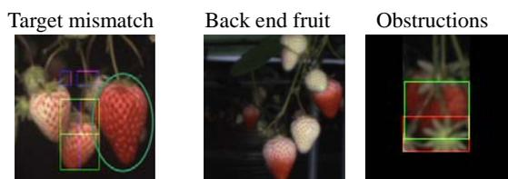
Fig. 8 Target detection failure
