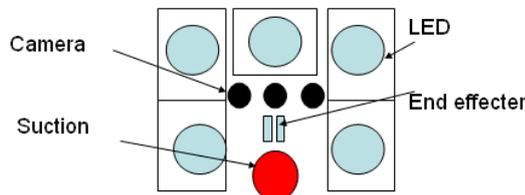
Fig. 2 Light source and camera layout
